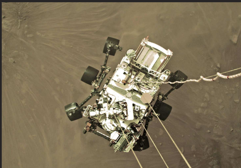
T aken from the descent stage, a snapshot of Perseverance rover from about two meters above the Martian surface. This image was sent down the coiled umbilical into Percy for later transmission before the descent stage disconnected from the rover and flew off to a safe distance. [NASA/JPL-Caltech]
